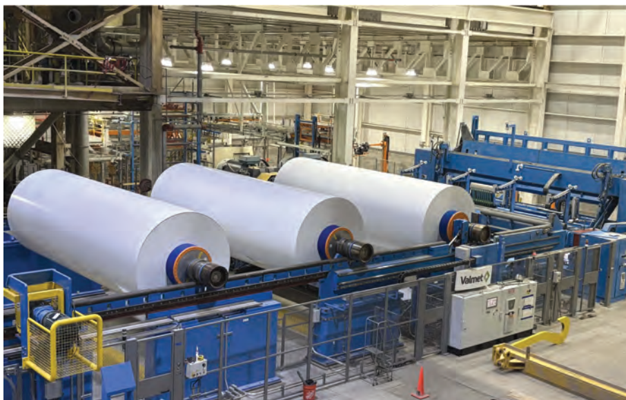
As production continues to ramp up, PM2 is planned to deliver 520,000 short tons per year (approximately 470,000 metric tons) of SBS paperboard grades, including folding carton, food service board, and cups.
