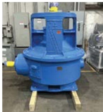
Rebuilt Black Clawson #4 Hydrapulper Drive Gearbox.
