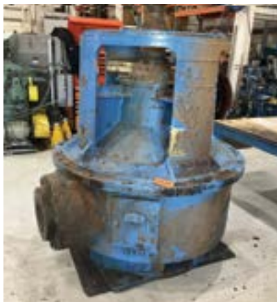
Black Clawson #4 Hydrapulper Drive Gearbox before rebuild.
