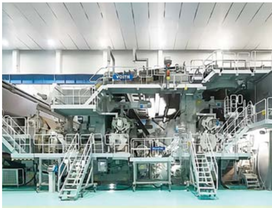
The Tandem NipcoFlex (pictured above) provides a good example of how NipMaster works. For an optimal configuration, precise drainage distribution between the first and second nip is crucial.
