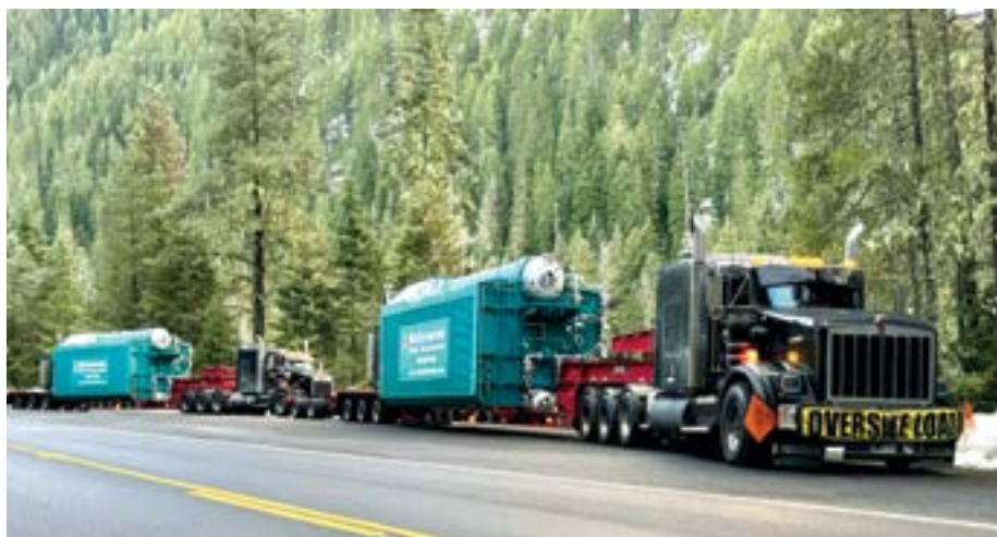
Two package watertube rental boilers in route for a temporary rental project.
