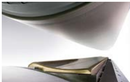
The design of the NipcoFlex shoe with top and bottom parts in combination with an insulation leads to low bending, excellent line load profiles and reduced maintenance effort.
