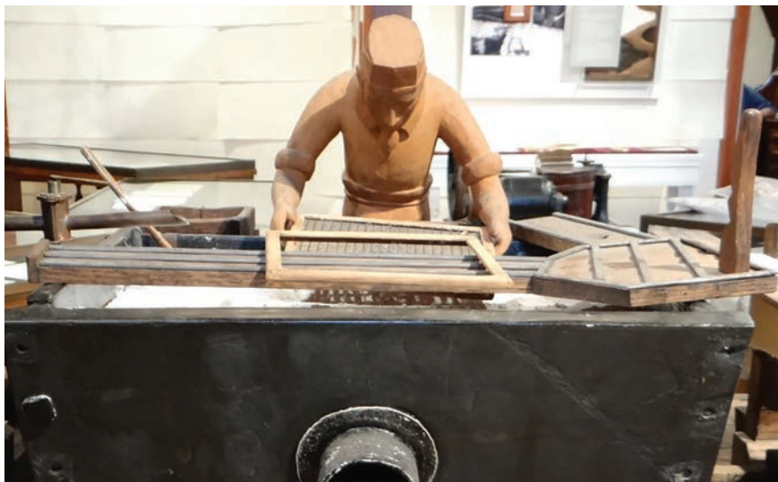
Vatman. Of the three major jobs in the mill, the Vatman was the real artisan. He would dip his mould, a framed wire screen, into a vat of liquid pulp or "stuff" and lift out a layer of fibers that would become a sheet of paper. The layer of fibers was laid between felts and then placed on a press. After the water was squeezed out, the paper was hung over ropes to dry. Image from the Crane Museum, Dalton, Mass.
