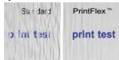
Figures 9-12. From a comparison of standard press fabrics and PrintFlex P (Figure 9), results taken from paper made in commercial trials has confirmed that a reduced fiber impression within the press nip (Figure 10), contributes directly to a smoother sheet surface profile (Figure 11) and a significant improvement in measured printability (Figure 12).
