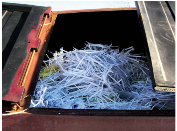
The recent trend of shredding recovered papers, such as mixed office paper, is allowing contaminants, especially stickies, to more easily enter the recycling process.
