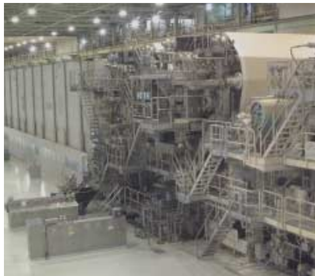
Miramichi's PM 2, one of the most modern magazine paper machines in North America. Miramichi mill produces 450,000 tpy of coated magazine paper.
