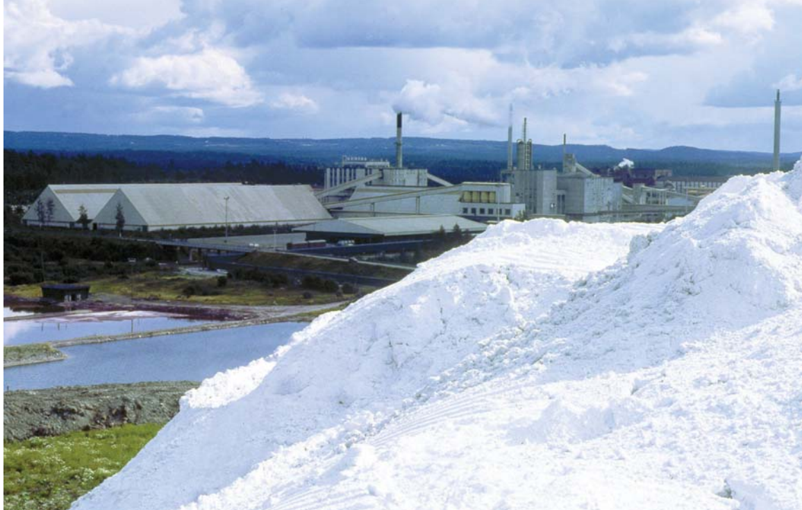
Kemira uses the by-product gypsum produced at its Siilinjärvi phosphoric acid plant as the raw material for its calcium sulfate pigments.
