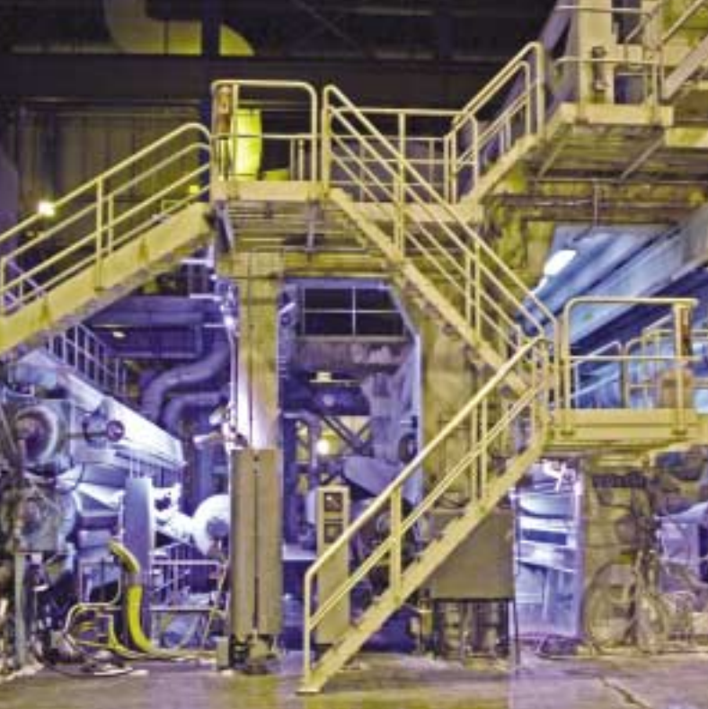
PM 26 two-roll machine calender (left) and the first of two rebuilt, online short-dwell coaters (on right), one for each side of the sheet.
