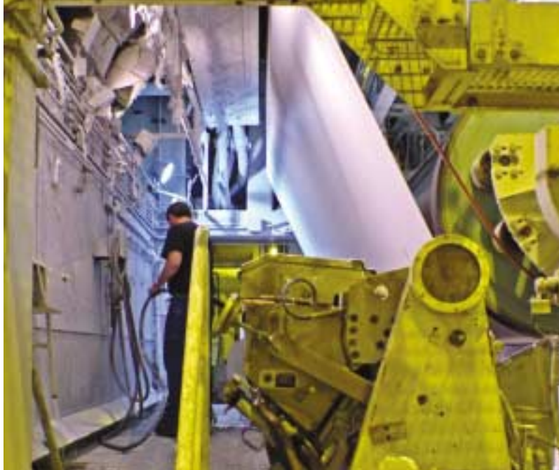
Both on-line coaters received new short-dwell coating heads in the Phase II rebuild, and the coating color delivery system was upgraded for faster, more reliable delivery.
