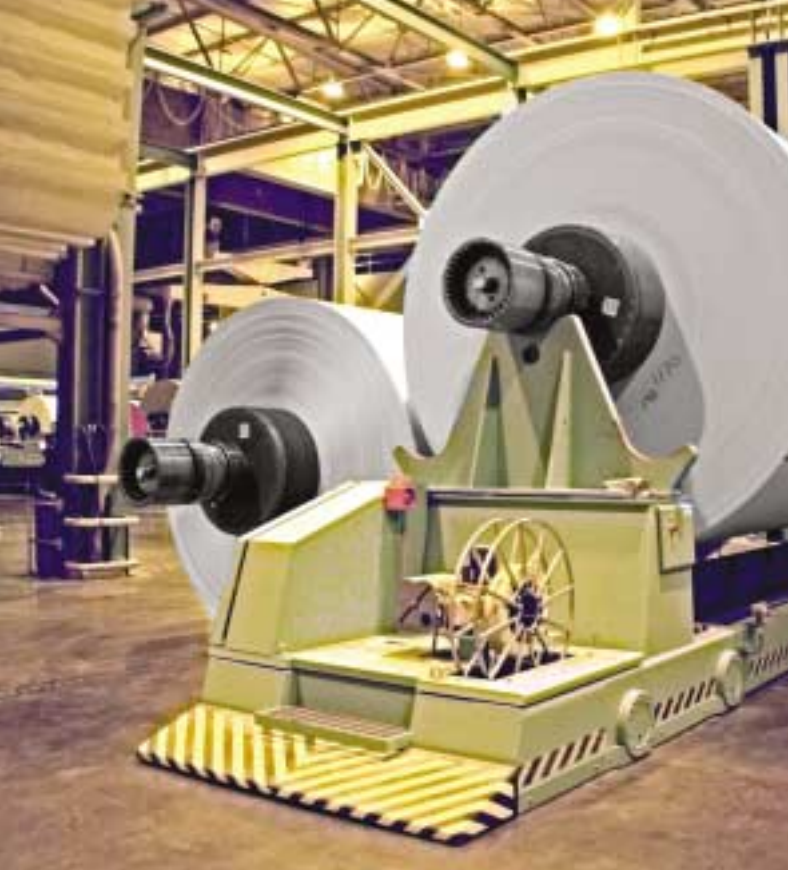
New parent reel carts operate between the re-reeler and the calenders, and between the calenders and winders.
