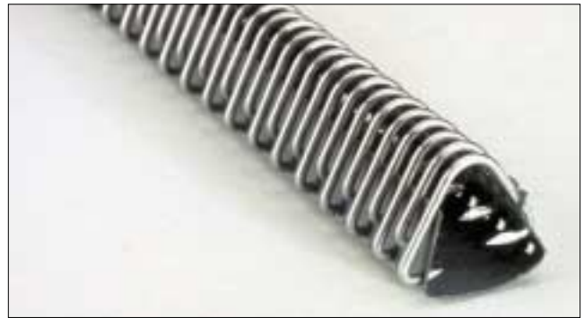
Figure 2. A carded assembly holds individual wire hooks together and is subsequently removed after splice installation.
