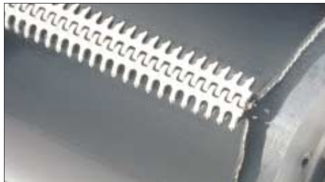
Figure 6. Stamped metal tooth fasteners require no specialized installation tooling.
