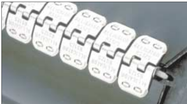
Figure 4. Hinged-plate fasteners provide extra holding strength due to upper and lower fastener plates that sandwich the belt ends and the use of dual staples.
