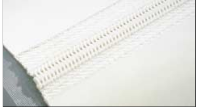
Figure 9. The plastic spiral fastener has a very low profile and can operate over small pulley diameters.
