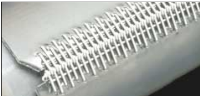
Figure 1. Wire hook mechanical fasteners are both economical and long lasting.
