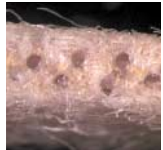
Figure 3. Filler material (yellow) trapped within the base fabric
