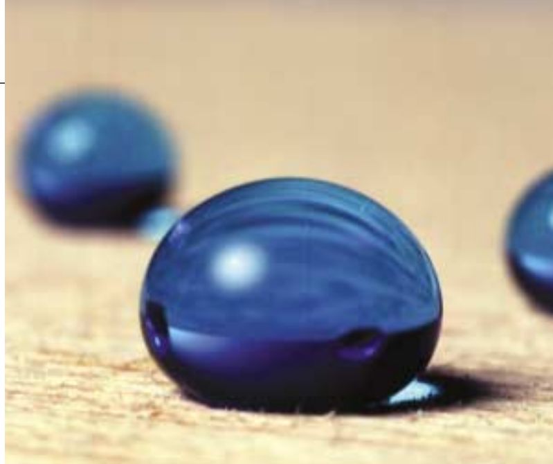
Water droplets rest on a wood surface impregnated with a nanoparticulate surface coating, making the surface extremely water-repellent (superhydrophobic). The coating also decreases the forces of adhesion, making the water droplets assume a globular form. Photo courtesy BASF.
