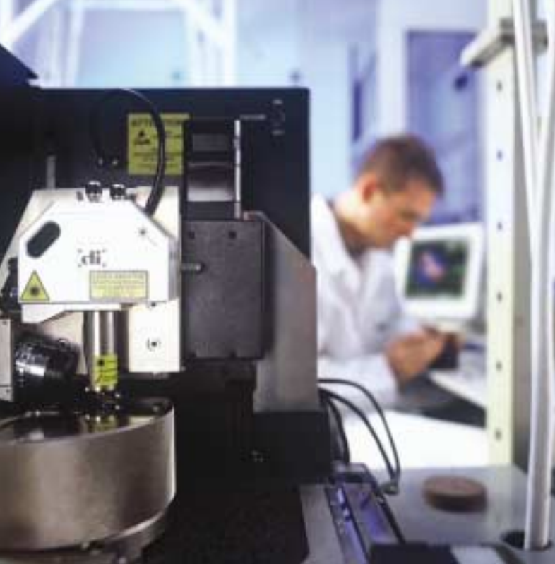
A frequently used method of nanoanalysis is atomic force microscopy (AFM), by which the surface of a sample can be analyzed with nanoscale resolution. Photo courtesy BASF.
