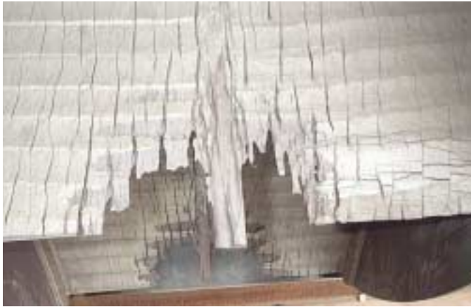
Figure 2. Fan blades protected by chrome carbide weld overlays after 12 months in operation.
