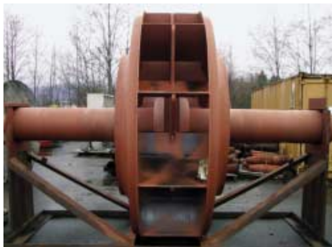
Figure 1. Port Alberni's power boiler ID fan.
