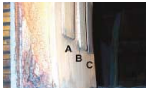
Figure 4. Comparison of material lengths after six months: (A) alloy steel, (B) chrome carbide weld overlay, (C) brazed tungsten carbide cladding.
