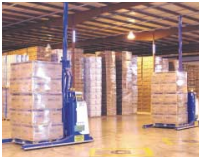
The 40-plus AGVs by Rocla/Swisslog are guided by control transmitters in the ceilings. These fully automated units are unmanned, self-charging, and completely maintenance free.
