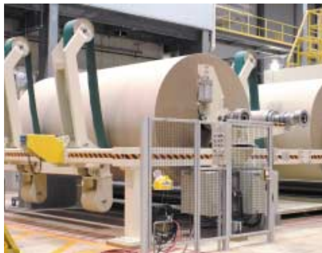
Parent rolls for brown and white napkin and towel products are produced on the new machine from a 100% recycled furnish processed using a state-of-the art Voith Andritz flotation deinking line at the complex. (Photos in this article courtesy of SCA/Patrick Hood).
