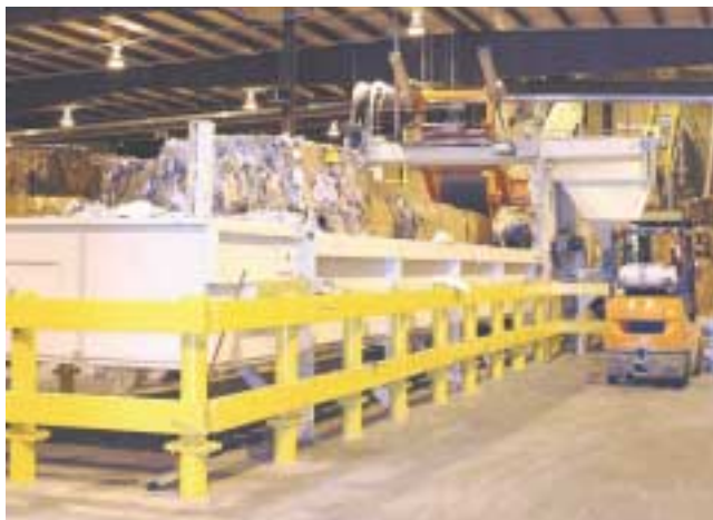
The mill's deinking line processes some 140,000 tpy of OCC, residential mixed papers, sorted office papers, and coated book stock.
