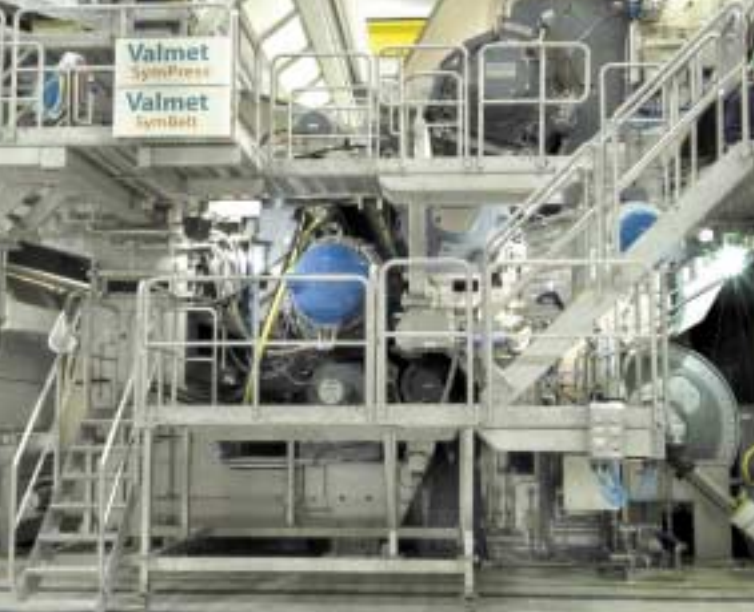
The three-nip SymPress B press section includes a SymBelt shoe press in the third nip. The section is equipped with a steam box located against the press suction roll and an IQMositure CD control package.
