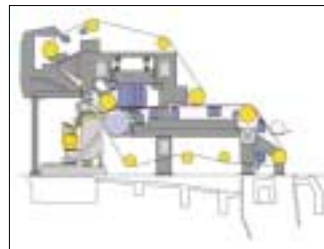
Figure 3. Generally, gap formers can be installed on existing fourdriniers as horizontal gap formers, or existing gap formers can be retrofitted with the key components of a roll-blade gap former to improve paper quality.
