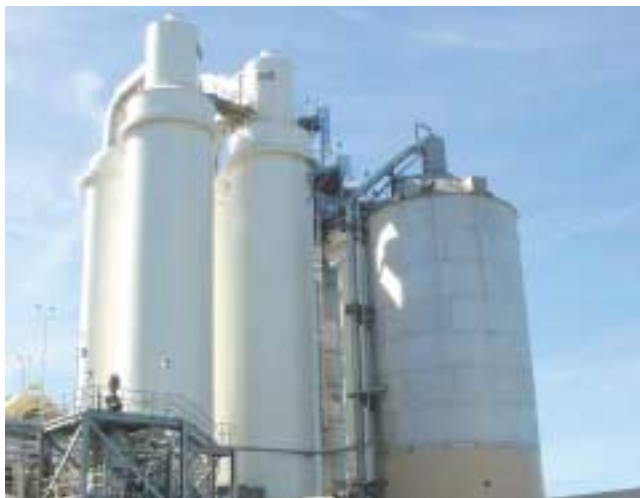
The ECF bleach plant has a DE op DD sequence with washing between the last two dioxide stages.
